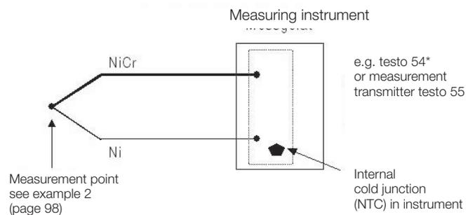
\* In testo 54 (external process display), the cold junction temperature can be read when the TC input is shorted.
