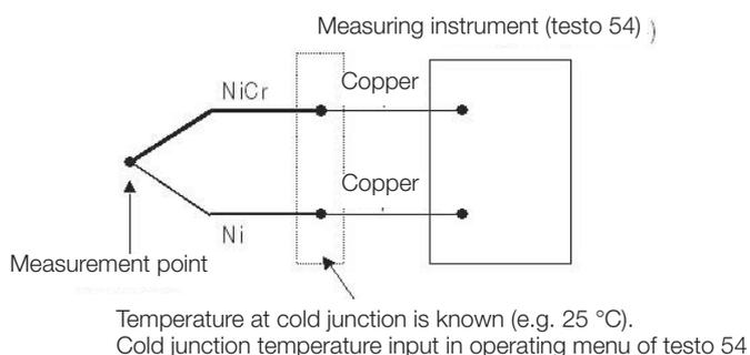
Correction of standard basic values (cf. chap. C 15), when the cold junction temperature deviates from 0 °C (examples):
