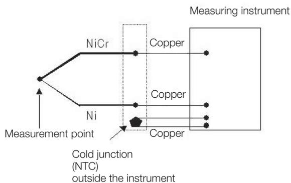
**External cold junction in testo 54 with any material (e.g. copper)**
