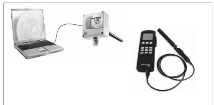
III. 1-point adjustment with the reference measuring instrument and the P2A software.
