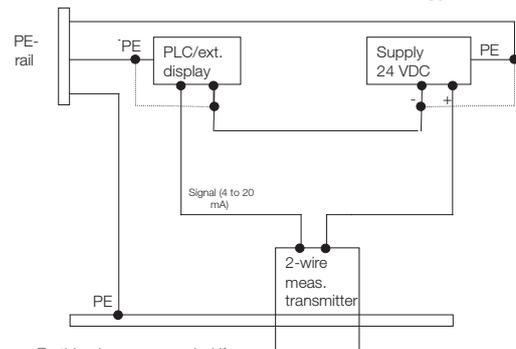
Earthing is recommended if potential differences exist between measurement location (e.g. container wall) and voltage supply/external display/PLC
