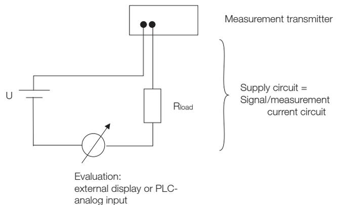
The maximum load shows how high the permitted total resistance of the instruments connected in the circuit (without the measurement transmitter), and the installed wiring, can be. The sum of the resistances may not be higher than the maximum load.
