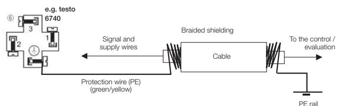
**6. Connect PE (protection wire) with low impedance (low resistance)**
