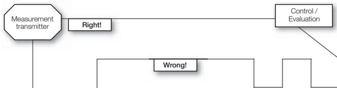
**2. Measurement transmitters and measurement displays may not be installed directly adjacent to guards, mains switches, motors, frequency converters and similar**
