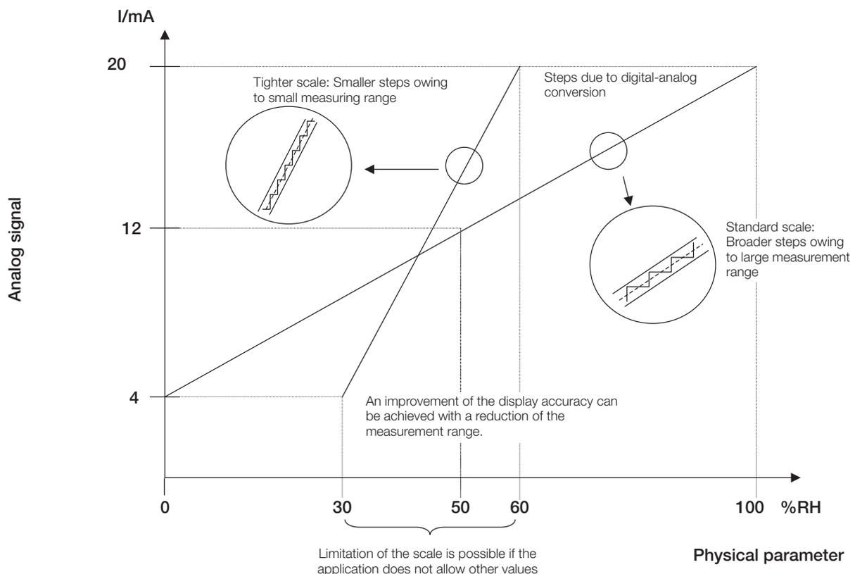
The diagram shows two different measurement transmitter scales, 0 to 100 %RH and 30 to 60 %RH. The resolution of the current signal remains constant (the number of steps), which is why the steps are compressed when the scale is reduced horizontally.
