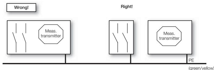
**3. Screening units should always be used on guards and other switching equipment**
