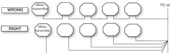
**8. When connecting the protection wire to (metal) measurement transmitters, ensure that the transition resistances are as low as possible**
