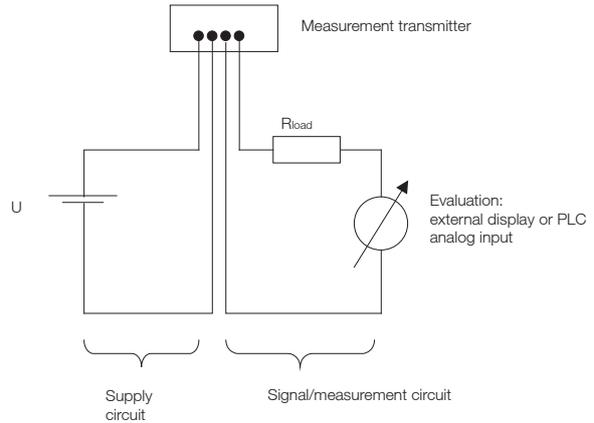
The maximum load shows how high the permitted total resistance of the instruments connected in the circuit (without the measurement transmitter), and the installed wiring, can be. The sum of the resistances may not be higher than the maximum load.
