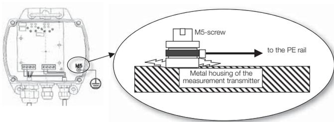
**9. Mutual zero potential is recommended if potential differences exist between measurement location (e.g. container wall) and voltage supply/external display/PLC.**
