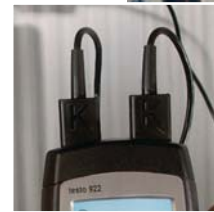
Simultaneous recording of temperature by two connected probes and display of differential temperature
