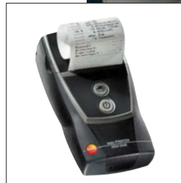
Print readings on site on testo printer
