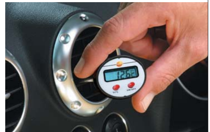
Measurements on air conditioning units
