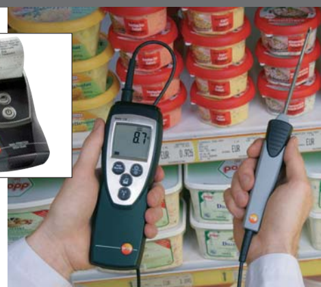
Inspects a refrigerated counter for sufficient refrigeration power
