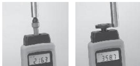
Mechanical with probe tip
