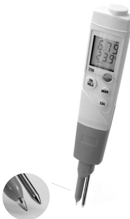
pH2 probe head for semi-solid food
