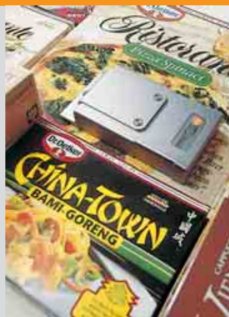
testostor 171-0 monitors fluctuations in temperature constantly
