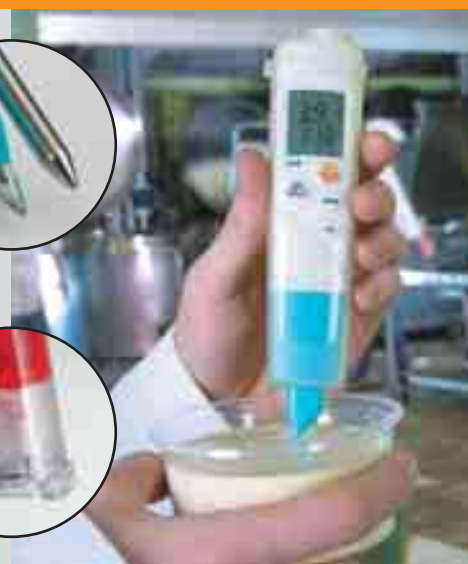
Spot pH checks during the production of dressings
