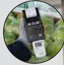
testo 177-T2 with display, data is printed on the fast testo 575 printer
