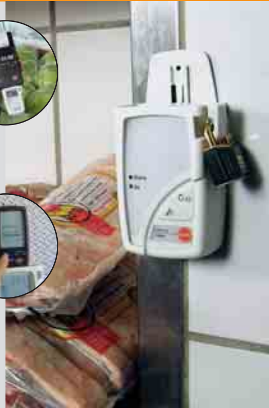
Long-term temperature logging in an intermediate store with testo 177-T1 (without display)
