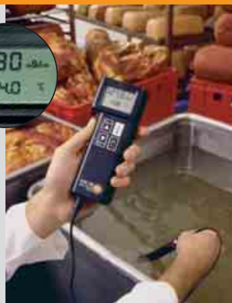
Measuring salt level (NaCl) in pickling brine
