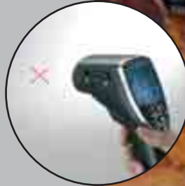
Switch optics 1: Far-field 75:1 (16 mm, distance 1200 mm) with cross laser marking
