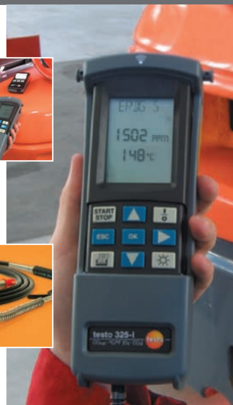
Tuning motors with the CO high [O 2 ] analyser
