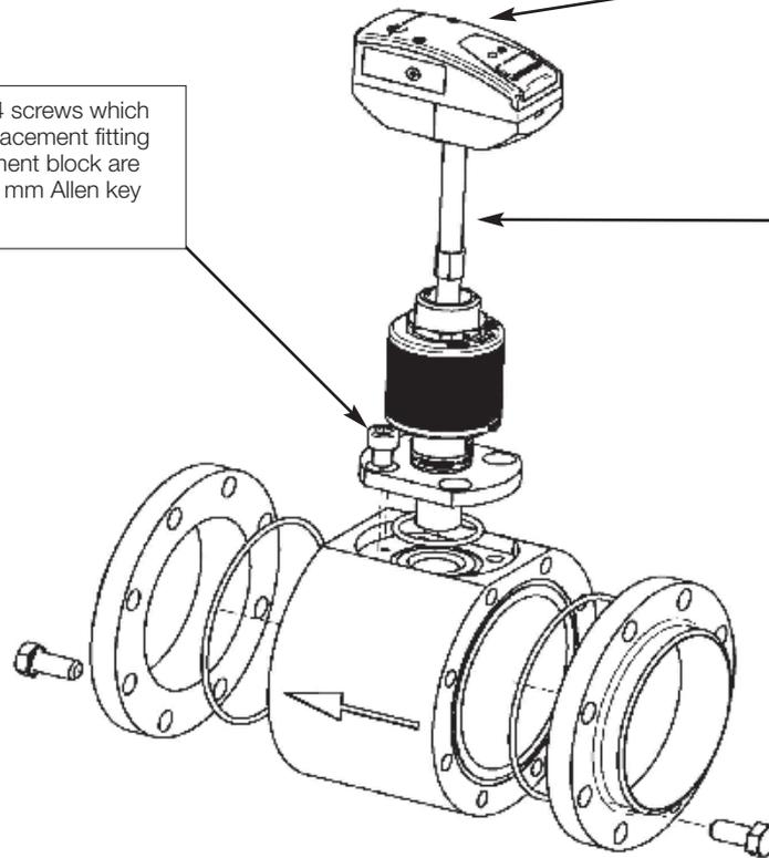
Then turn the replacement fitting to the position CLOSE by hand. This means that the replacement fitting is sealed to the interior of the pipe.
