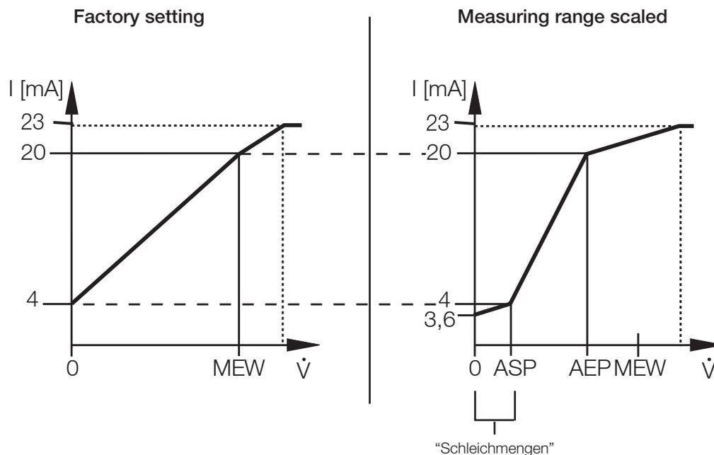
**Application:** Leakage detection (limit value monitoring via PLC) or consumption quantity measurement (integration via PLC)
