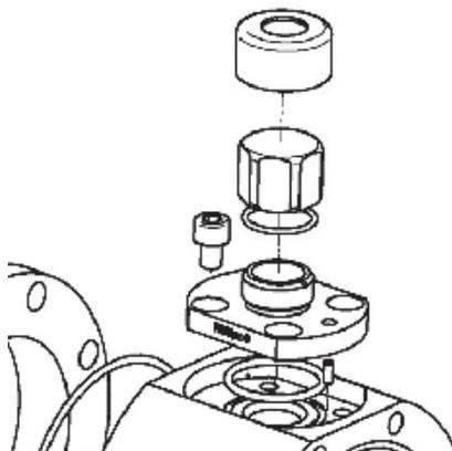
The sealing cap must be ordered as an accessory, it is not included in delivery.
