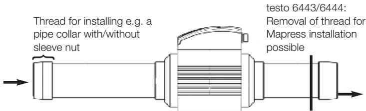
Install the testo 6440 in such a way that the the flow direction and the marking arrow are pointing in the same direction.
