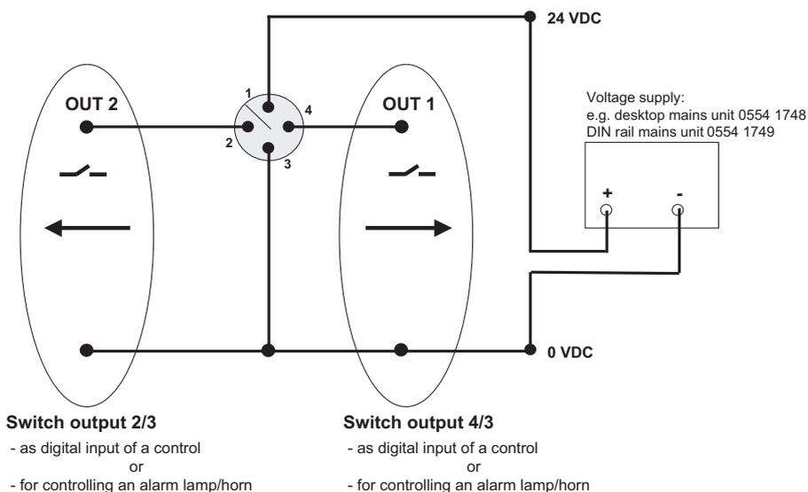
**Wiring testo 6441...6447 alternative B**
